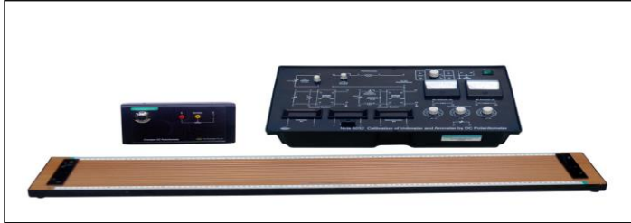
Calibration of Voltmeter using Potentiometer
